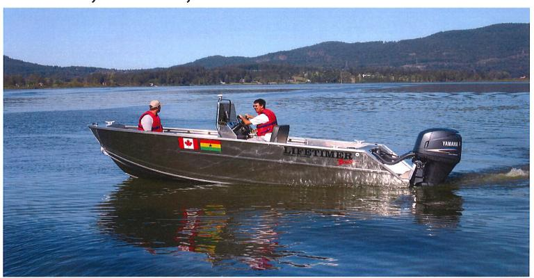
The big, beamy Offshore models with their optional center console steering and roomy interior make an ideal craft for fishing on lakes, coastal and open waters. Like all Lifetimer boats, they are built to move fast and safely in the most adverse of weather and water conditions. Our tapered delta-planing hulls with reverse chines and sharp, deep bow entry are one of the driest, safest and most seaworthy boats on the market today.
